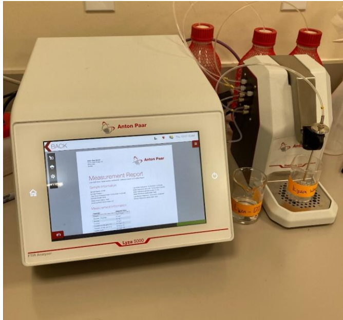
Figure 26. Anton Paar Lyza 5000 Wine Analyzer. The Analyzer can measure 19 parameters in approximately 3 minutes per sample.
