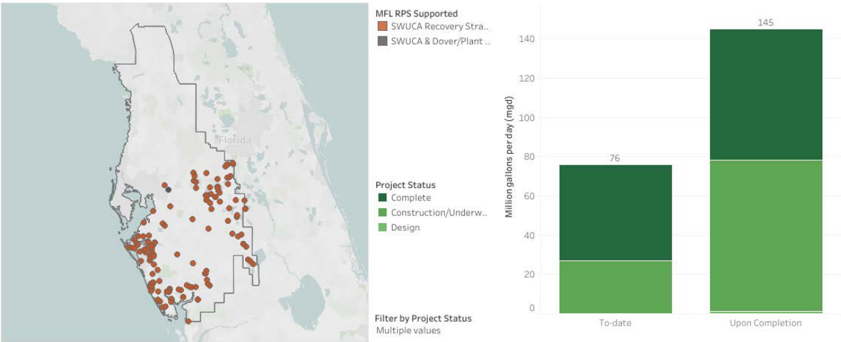
Figure 70. Map of SWUCA Recovery Strategy projects designed to achieve the MFLs and graph of water quantity benefits from projects
