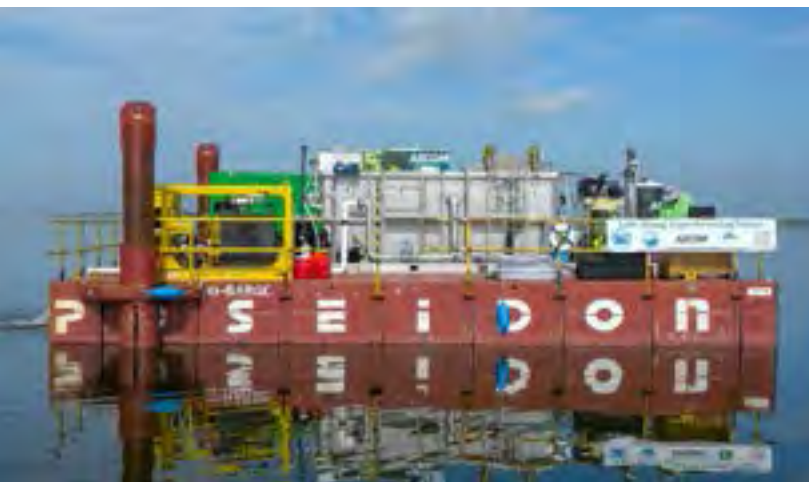
A mobile algal harvesting unit mounted on a barge was used to remove algae from Lake Jesup in a pilot project.
