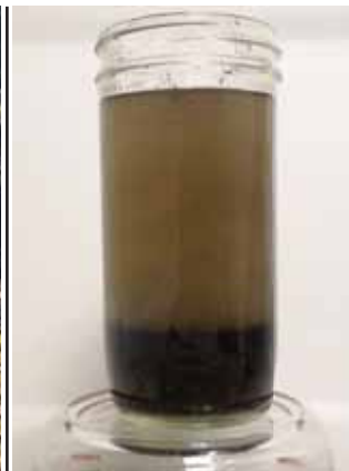
The heavier sands fall out almost immediately. The lighter muck molecules will fall out over time and drop into the bottom of the dredge material management area.
