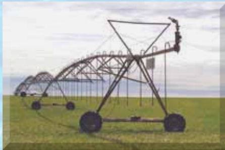
Radial Pivot Irrigation
