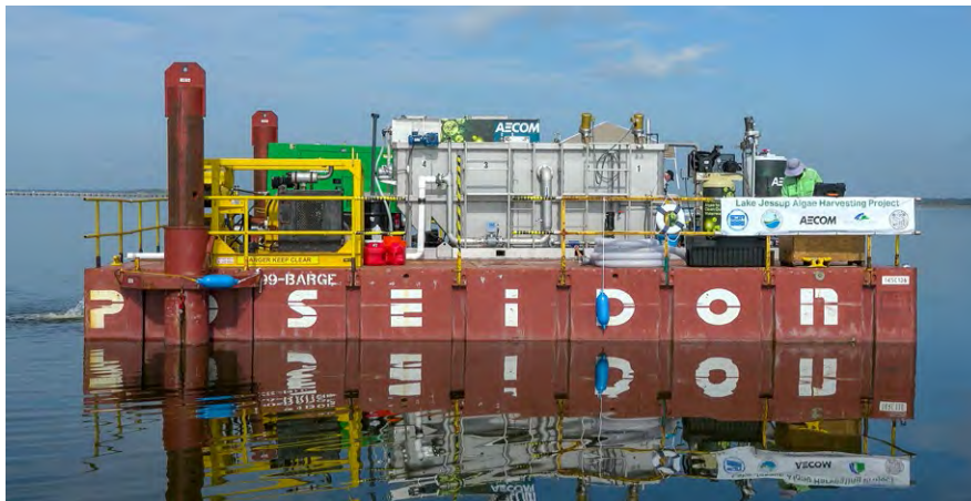
A mobile algal harvesting unit mounted to a barge remove algae from Lake Jesup during a pilot project.
