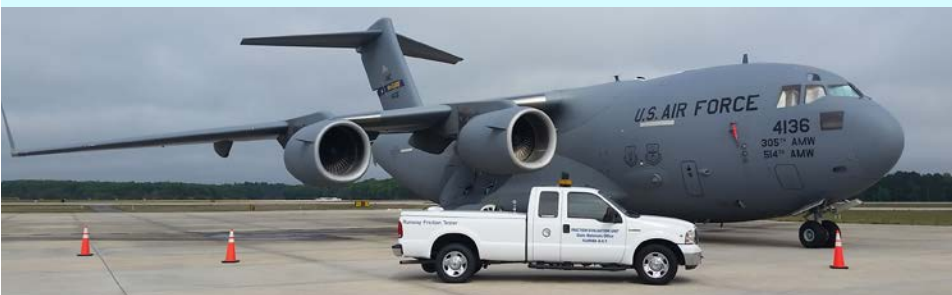
To ensure the safety of the traveling public, approximately 8,000 lane miles of the State Highways System and runways of 25 major airports are evaluated on an annual basis with a specialized friction unit pictured here.
