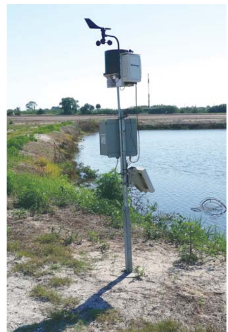
Weather station in Hillsborough County.
