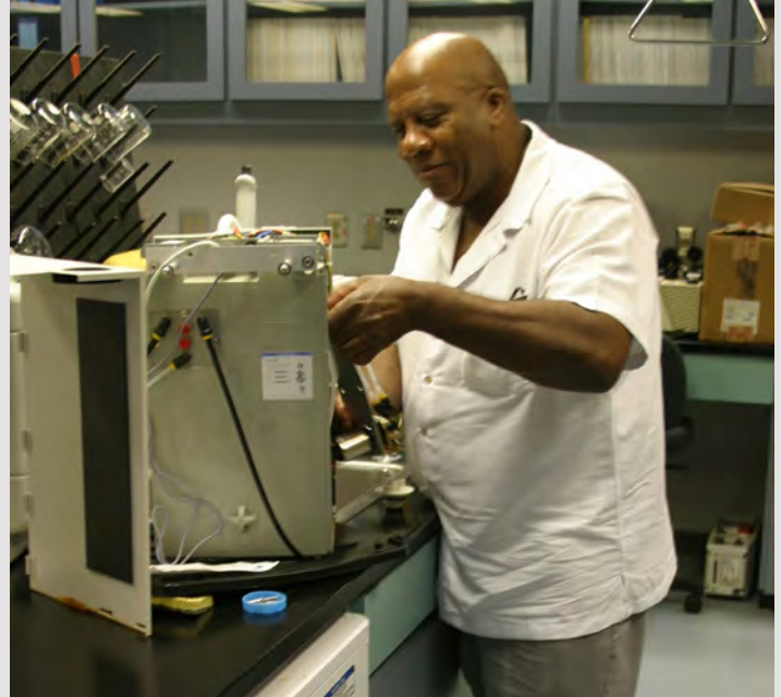
Maintenance Superintendent, Lynn Lee repairing the Water Deionizer used for Explosives Analysis
