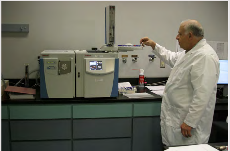
Analyst Sam Blittman placing vials of extracted fire debris on the GC-MS for analysis
