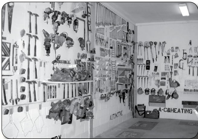
When inmates use tools in the course of their job in a prison, they have to check them in and out daily. This crude but effective inventory system, where a picture of the tool is painted on the wall, allows correctional officers to see at a glance if a tool is missing and who has it. This method is also used for kitchen utensils.
