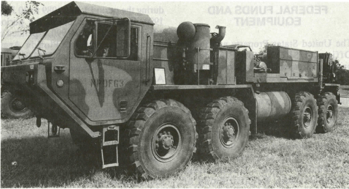
The HEMMET truck serves as a heavy multipurpose workhorse including dump and tanker trucks. Shown here is the HEMMET wrecker.
