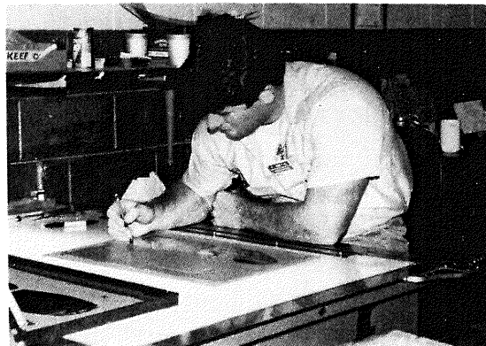
Image assembly, or stripping, is a pre-press function requiring a high level of awareness and skill. Here, the film negatives are stripped into precise position for burning of the image onto an offset-press plate.
