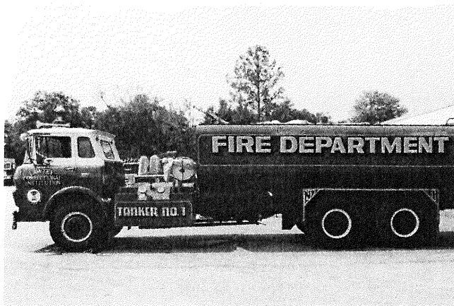
The 5,000 gallon tank truck also stationed at the Lawtey C.I. Fire Department.
