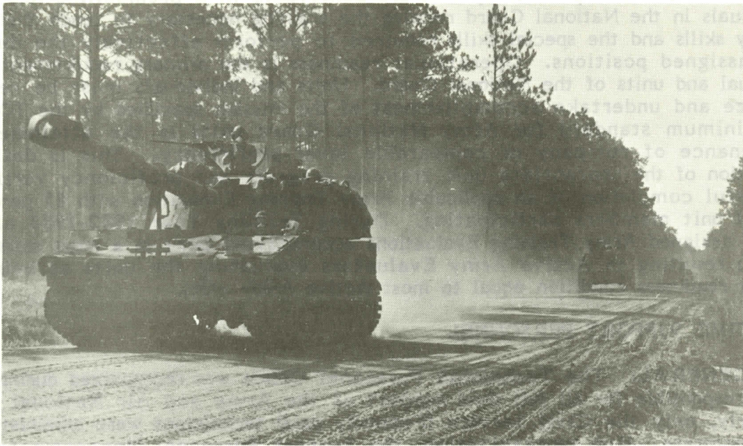
M109 155mm self-propelled howitzers move out during annual training at Fort Stewart, Georgia
