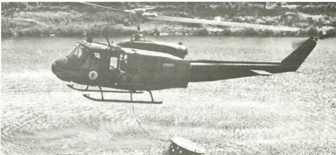
Florida Army National Guard Huey Hovers Over a Water Supply While 400 Gallon Water Bucket Fills
