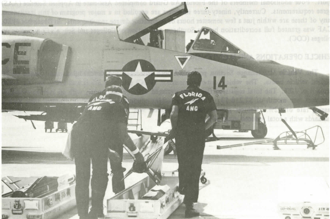
AIM Missiles Being Loaded Onto a Florida Air National Guard F-106 by Florida's Champion Loading Team
